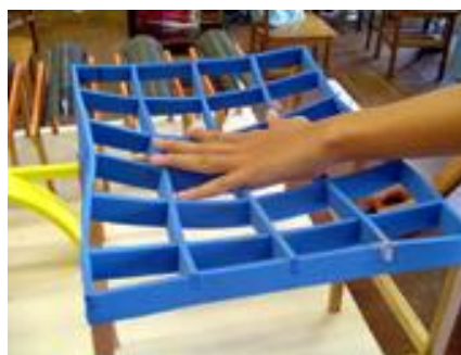
Figura 2.17 – Laje nervurada (grelha)
